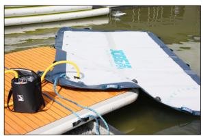
Place the corner where the valve is located onto the transom of your boat. Make sure it doesn't float of the transom in the next step.
