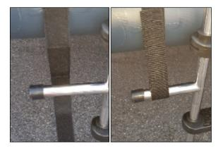
Place the straps onto the ladder like the below photo. Adjust the straps if needed.
